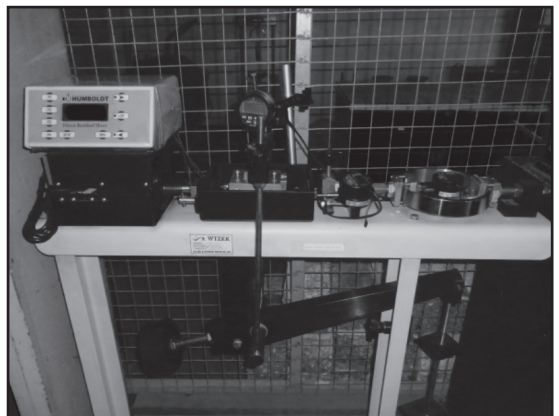
Digital Direct shear apparatus for testing soil shear strength
